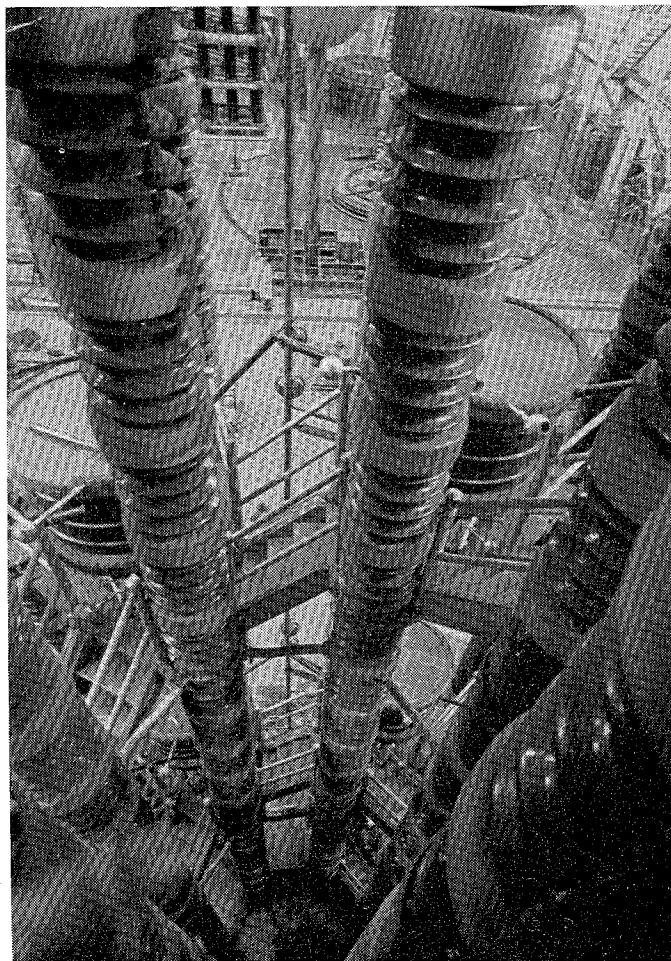
Science promises great things for the future and Soviet scientists are well to the fore. Right: insulators of the test equipment which can produce "lightning" of 7,300,000 volts. Note the size of the two scientists in white overalls.
