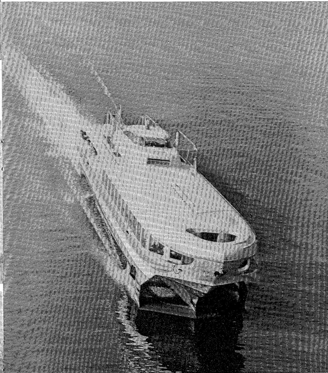
The hydrofoil principle is being extended at Red Sormovo to larger vessels. The sixty-seater shown here has given a good account of itself and many others are to be built for fast transport on the Volga.
